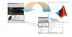
Just a few source code lines in WinTAX4 allow the content of the Matlab<sup>®</sup> workspace to be displayed without loading logged laps  $\rightarrow$  WinTAX4 becomes a Matlab displayer.
