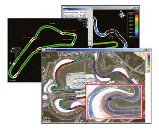
*Track values:* values of channels are displayed together with cursor when moving.
