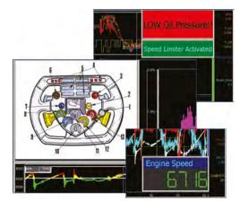
The Bitmap Window allows you to insert one or more images into WinTAX layouts. Standard Jpeg, Bmp, PNG and GIF files are supported.
